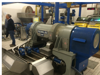
Pieralisi "decanter" is a centrifuge efficiently separating oil from water and organic matter.
