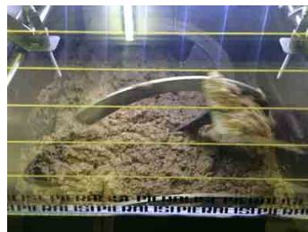
Olive Pate' malaxing Releases oil from paste
