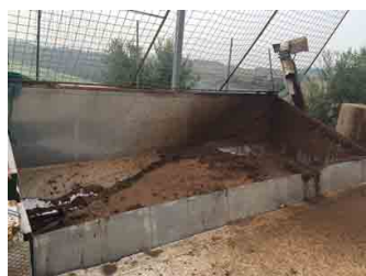
Olive waste is fed into olive pit processor below
